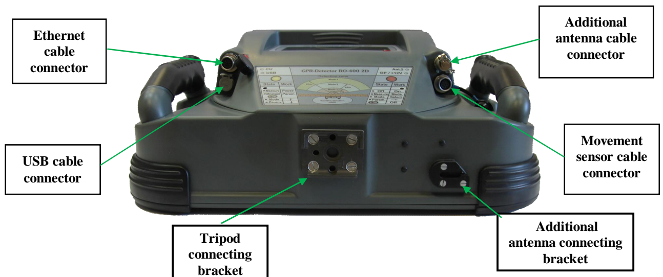
Fig. 5.2. Arrangement of sockets to connect cables to GPR detector
