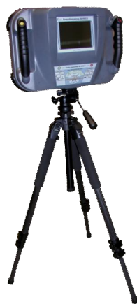
Fig. 5.4. GPR detector secured on the tripod
