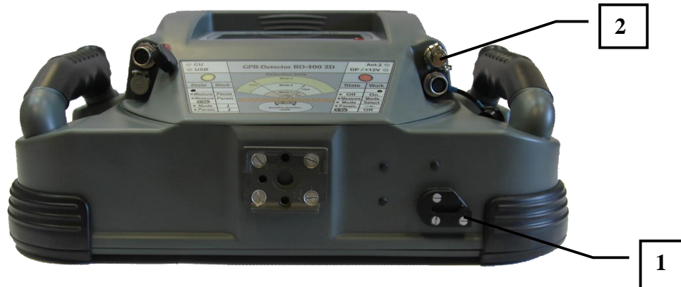
Pic.6.1. Antenna Unit RO-4002D with additional antenna unit
